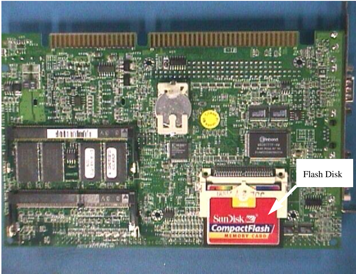
Figure 2-4: Location of Flash Disk on the NXG Microprocessor Board
