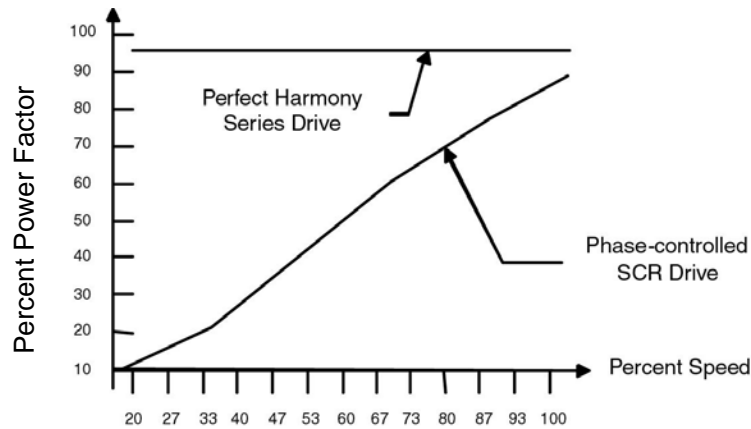
Figure 1-2: Comparison of Perfect Harmony and a Typical Phase-controlled SCR Drive
